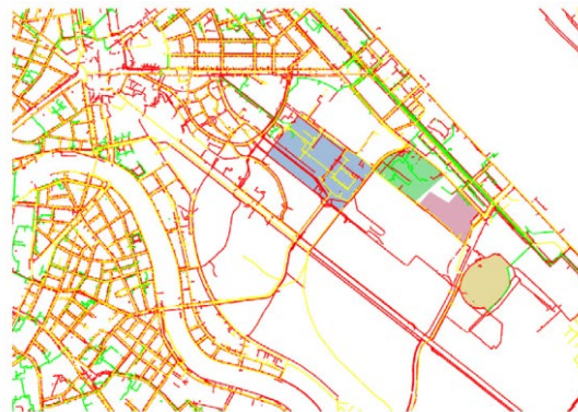
(d) Existing distribution grid of gas (yellow), district heating (green) and electricity (red) in the urban neighborhood and its surrounding area. Source: [47]
