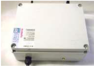
6 Figure A1 The sensor used to measure the indoor temperature: QC0160 ultra-RF, manufactured 7 by Invisible System Limited (7.5min data profile, accurate to \pm 0.5^{\circ}\text{C} ).
