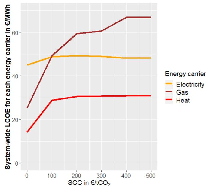
Figure 8 Average system-wide levelized cost of energy for each energy carrier in €/MWh<sub>e</sub> for electricity and €/MWh<sub>th</sub> for gas and heat
