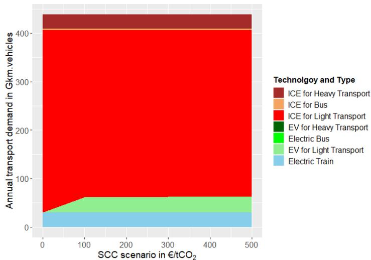
Figure 6 Transport supply by mobility type and vehicle technology type in Gkm.vehicles/year as function of SCC (the rail demand satisfied by electric train is expressed in TWh<sub>e</sub>/year)
