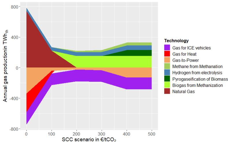
Figure 4 Gas production (positive) and its conversion to other sectors (negative) in TWh<sub>th</sub>/year as a function of SCC
