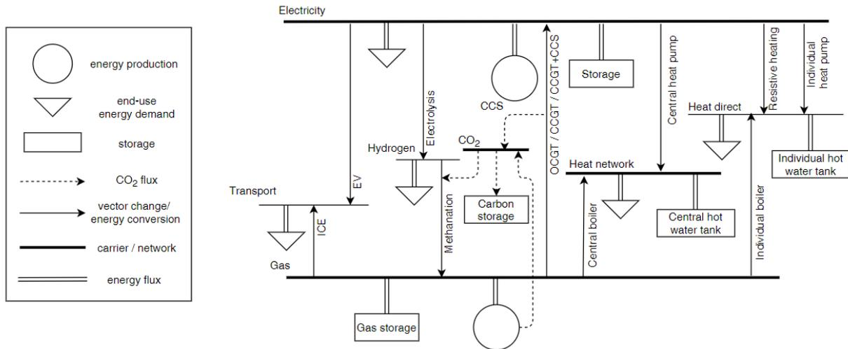
Figure 1 EOLES\_mv model representation; the figure at the right side shows the interactions between energy supply, demand, storage and carriers by energy flux and CO<sub>2</sub> exchanges. The box at the left side explains the meaning of each shape. The two energy supply technologies are electricity and gas production, each connected to its own network.
