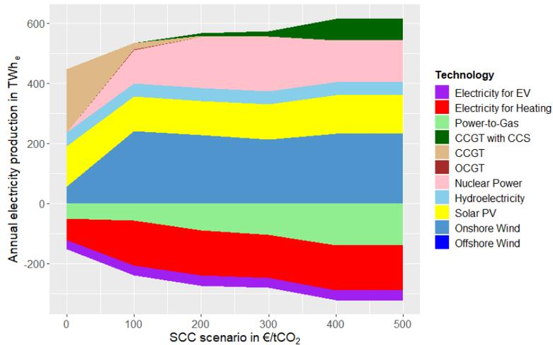
Figure 3 Electricity production (positive) its conversion to other sectors (negative) in TWh<sub>e</sub>/year as a function of SCC
