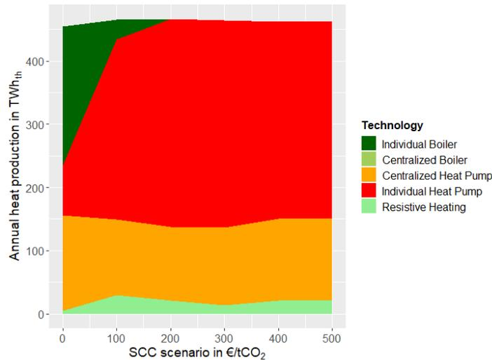
Figure 5 Annual heat production in TWh<sub>th</sub>/an as a function of SCC
