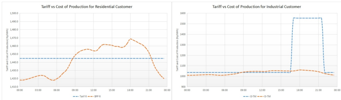
Figure 4. Tariff and cost of production for (a) residential customer and (b) industrial customer
