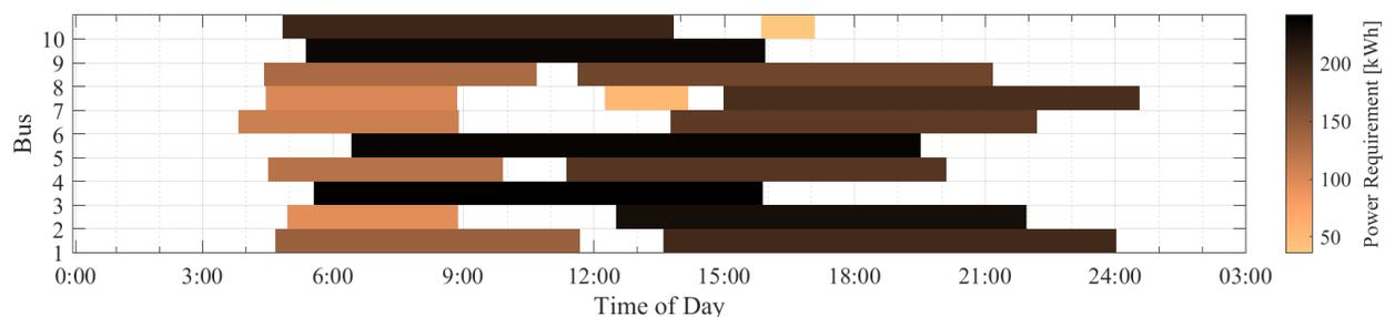
**Fig. 3: Resulting Cycle Sequence for ten 18-Meter Buses Using MILP-Solver. Total Mileage: 2277 Kilometers**
