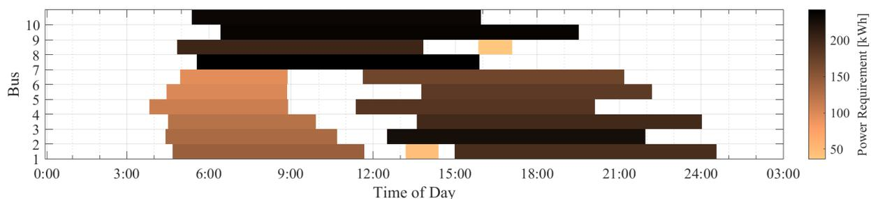
Fig. 2: Resulting Cycle Sequence for ten 18-Meter Buses Using the Algorithm. Sum Mileage: 2272 Kilometers
