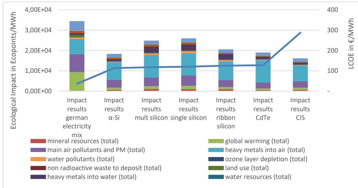
Figure 1 Ecological and economic comparison of the analysed photovoltaic systems
